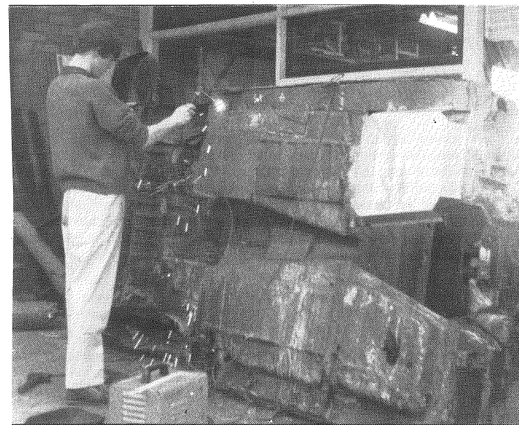
Fig. 3 Welding floor pan April 1983
